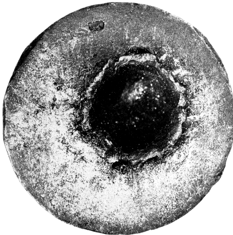
FIGURE 7. The deformation of a lead block caused by the impact of a 2 to 3 mm diameter water jet at a velocity in the range 1500 to 1800 m/s. Diameter of the depression 8 mm, depth 5 mm.
