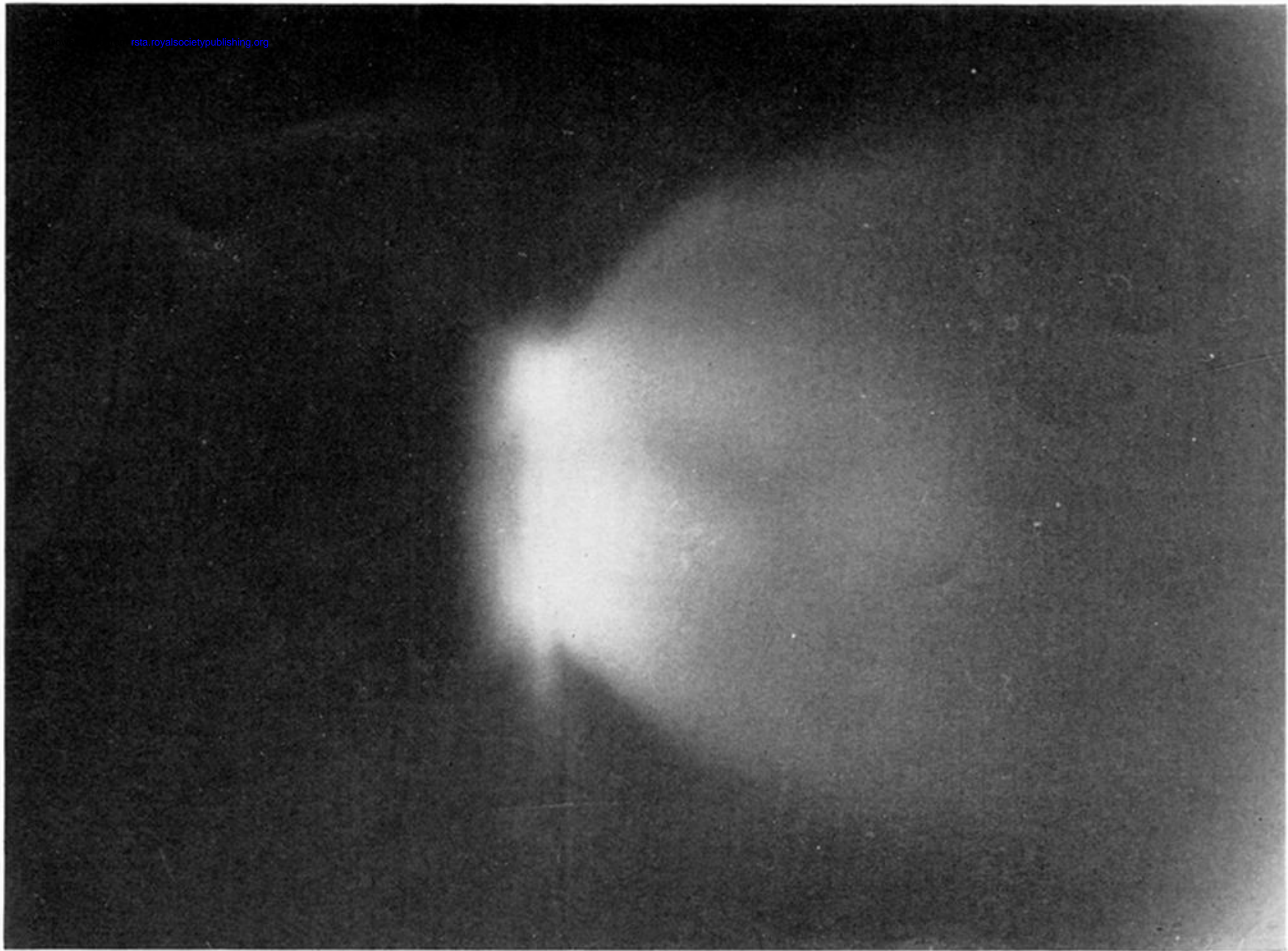
FIGURE 3. The light flash accompanying the impact of a water jet against a polymethylmethacrylate plate. Jet trajectory is horizontally across the figure from right to left.
